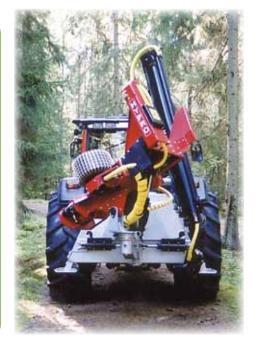
The HYPRO 755 is a generously equipped tractor-processor with a 7 metre crane. Processor and crane both have a working radius of 280 degrees, allowing felling on both sides.
