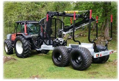
A Cranab FC53DT with lenght of 8,5 meters is used as crane option.
