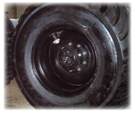
Hydraulic motor drive via planetary gear generates very strong work force. With the drive activated, the hydraulic motor has automatic free rolling up to 40 km/h with the LSsystem. The drive device is placed in the rear wheel pair.
