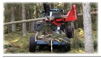
The **HYPRO 755 VB** is a trailer-mounted processor without crane, winch, pump or tank. It has been produced in order to combine a logging trailer with a crane and a processor, resulting in lower ground pressure and a lower purchase price.
