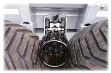
On the HYPRO HV14 you have the option of choosing between robson drive or planetary gear. HYPRO 4WD robson drive provides high drive power and the drive unit is well protected
