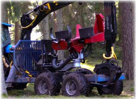
The processor is easy to mount directly onto just about any logging trailer using the trailer's own crane. The machine has three eye bolts, allowing it to be very simply and easily lifted using straps or chains. All hoses and cables do of course have quick-release couplings.
