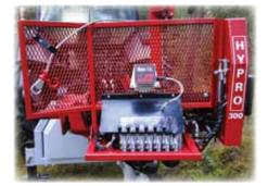
The machines control table is placed in a comfortable working height and has easily maneuverable levers, where it also is possible to adjust the speed in both directions individually on all functions. The measuring system is optimal placed for a comfortable use.
