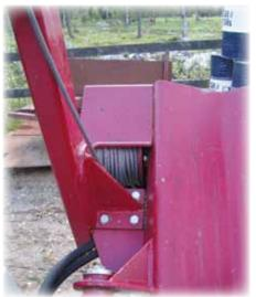
Hydraulic winch placed in the machine frame, maneuvered via radio or lever. At signal in / out the wire is fed in resp. direction and is always automatically locked at stop.
