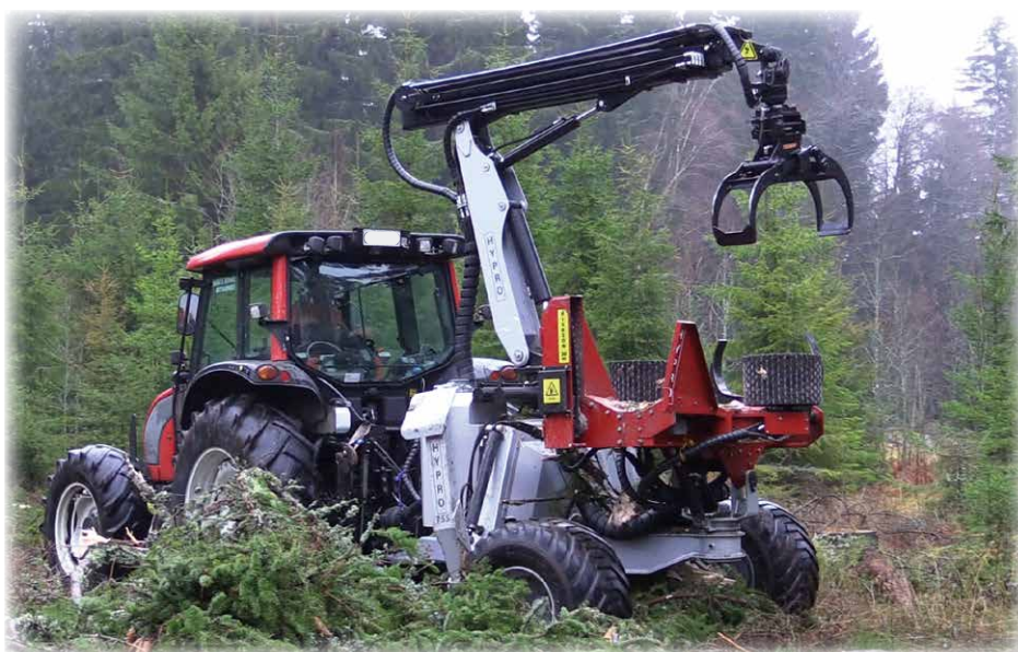
HYPRO 755 HB has hydraulic support legs and large 500/50-17 wheels as standard.
