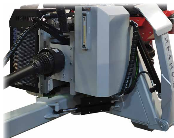
Articulated steering +/- 25° with double steering cylinders.
