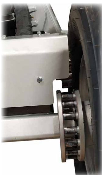
Articulated steering +/- 25° with double steering cylinders.
