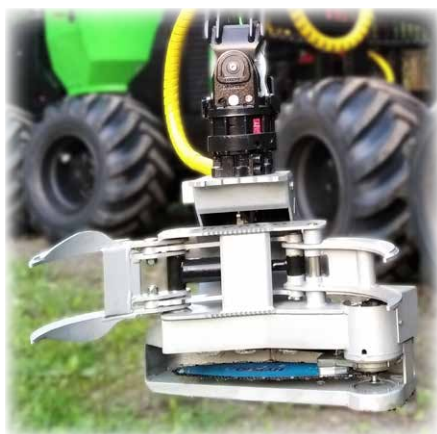
HYPRO FG45 can in principle be mounted on all cranes with rotators. The grapple opens about 92 cm and encloses down to Ø3 cm
